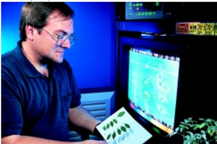
**Technician Wilbur Hershberger uses infrared thermography to evaluate the ability of water-repellent particle films to block ice formation in frost-sensitive plants.**
